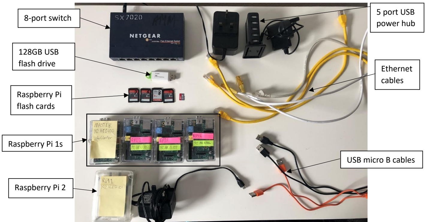
Figure 2 All hardware pieces use in the cluster.
