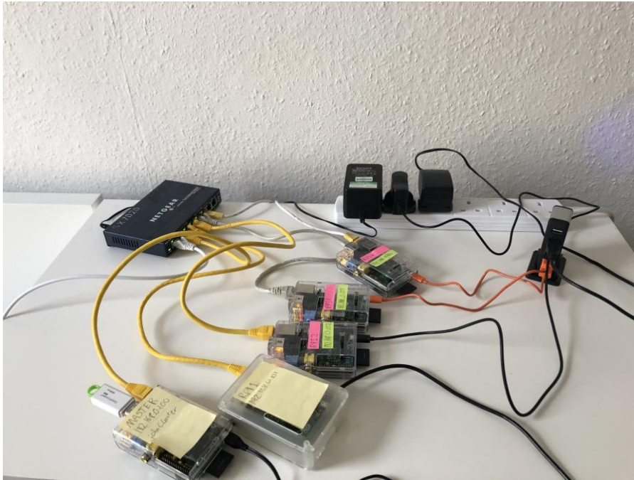
Figure 6 Pi cluster set up.
