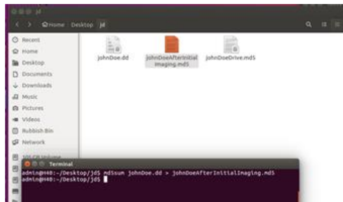
Fig 7 Creating the checksum
